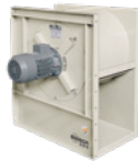
172 TCR/R/EW 400 °C/2h centrifugal extractor fans with backward curved impeller fitted with electronically adjustable, high efficiency, asynchronous IE3 motors
