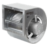
128 CJBD/EC/ALS Ventilation units with aluminum profile, double insulating wall and EC Technology IE4 motor with integrated electronics
