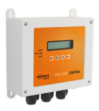
Control panel and independent automatic regulation for lobby pressurisation systems in accordance with standard EN 12101-6, compatible with systems KIT BOXPDS and KIT BOXPDS SMART acting as remote pressure sensor and with automatic damper control to maintain overpressure in lobbies in case of fire.
